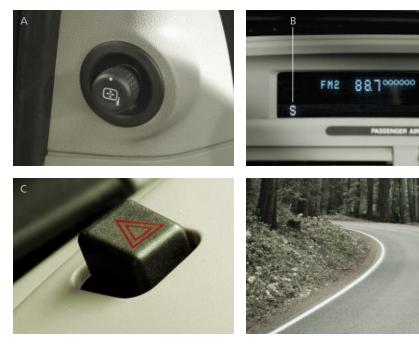
A. POWER SIDE VIEW MIRRORS – Rotate the control clockwise to adjust the right mirror, and counterclockwise to adjust the left mirror. Then move the control in the direction you wish to tilt the mirror. Return to the center position to lock the mirror in place.
